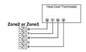
A heat pump thermostat can be used in Zone1 to provide emergency heat control from the thermostat. Be sure to set DIP switch #4 to HP.
