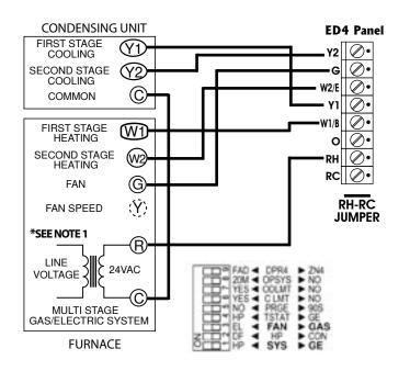
**\*NOTE 1:** Sometimes Y needs to be wired to the furnace for fan speed.
