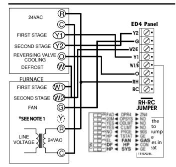
**\*NOTE 1:** Sometimes Y needs to be wired to the furnace for fan speed.
